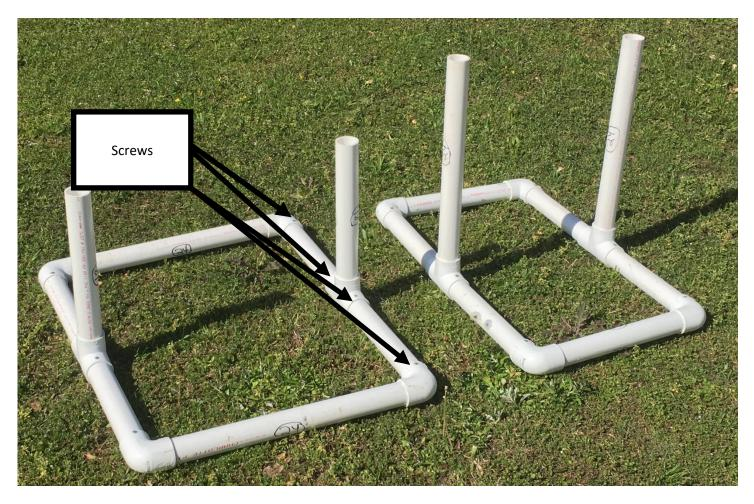
This assembly means that the front and rear sections and the uprights that hold the 1x2 can be easily swapped. If you need an IDPA stand, use the 14" sections for the front and rear sections and use the 20" section to hold the 1x2 furring strip. If you need to store the stand compactly, you can pull the sides off and remove the loose sections.
